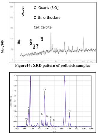
Figure15: EDX pattern of redbrick samples
