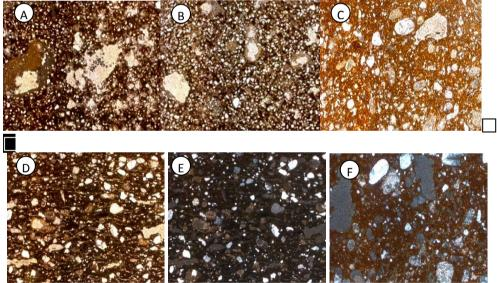
Figure 18: thin sections photomicrographs of bricks showing quartz grains, iron oxides, clay minerals and crystals of orthoclase 64 X.
