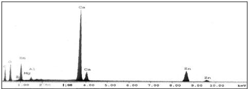
Figure21SEM-EDX spectrum of ground layer
