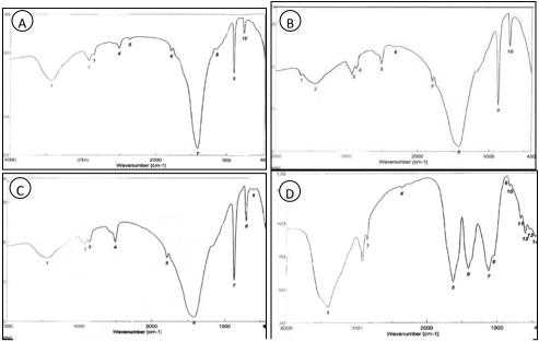
Figure22: FTIR spectra paint layer of St. George church dome A: blue pigment B: silver pigment C: gilded layer. D: Varnish layer.
