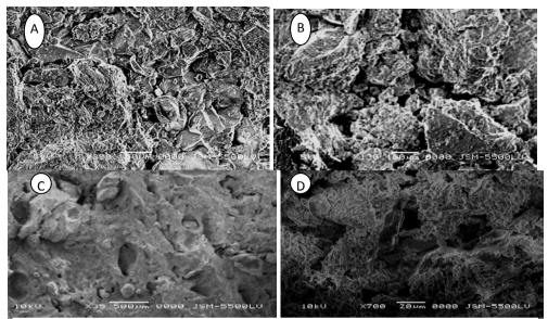
Figure 17: SEM photomicrographs showing the collapse of internal structure, voids, loose of binding material and salts crystallization between mineral grains.
