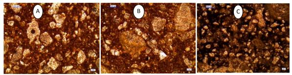
Figure16: optical microscope photograph of brick showing clay minerals, grain of quartz and iron oxide, also micro cracks, cavities and pits can be observed, 40-60x.
