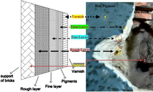
Fig.4 the mural painting structure layer **a**: plane of painting structure layer **b**: detail from area of loss on dome
