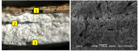
**Figure19:** LOM photograph of cross section stratigraphy of painted layer
