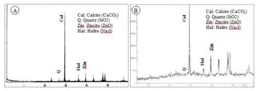
Figure20: XRD patterns of ground layer a: pattern of coarse ground layer b: pattern of fine preparation layer.
