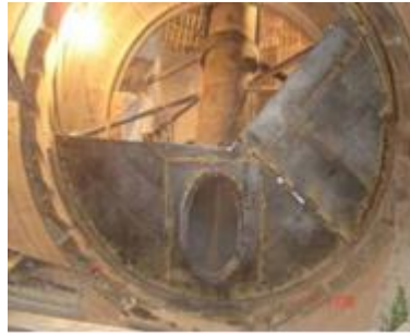
Fig. 2 Self-regulating continuous burden feeder
