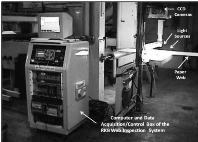
Figure 2. General view of the RKB web inspection system demonstration unit used in the pilot-scale experiments.
