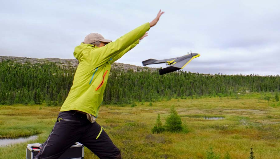
← UAV remote sensing for lake colour analysis and vegetation mapping near Kuujjuarapik (Nunavik, Quebec, Canada) © Ana Padeiro
