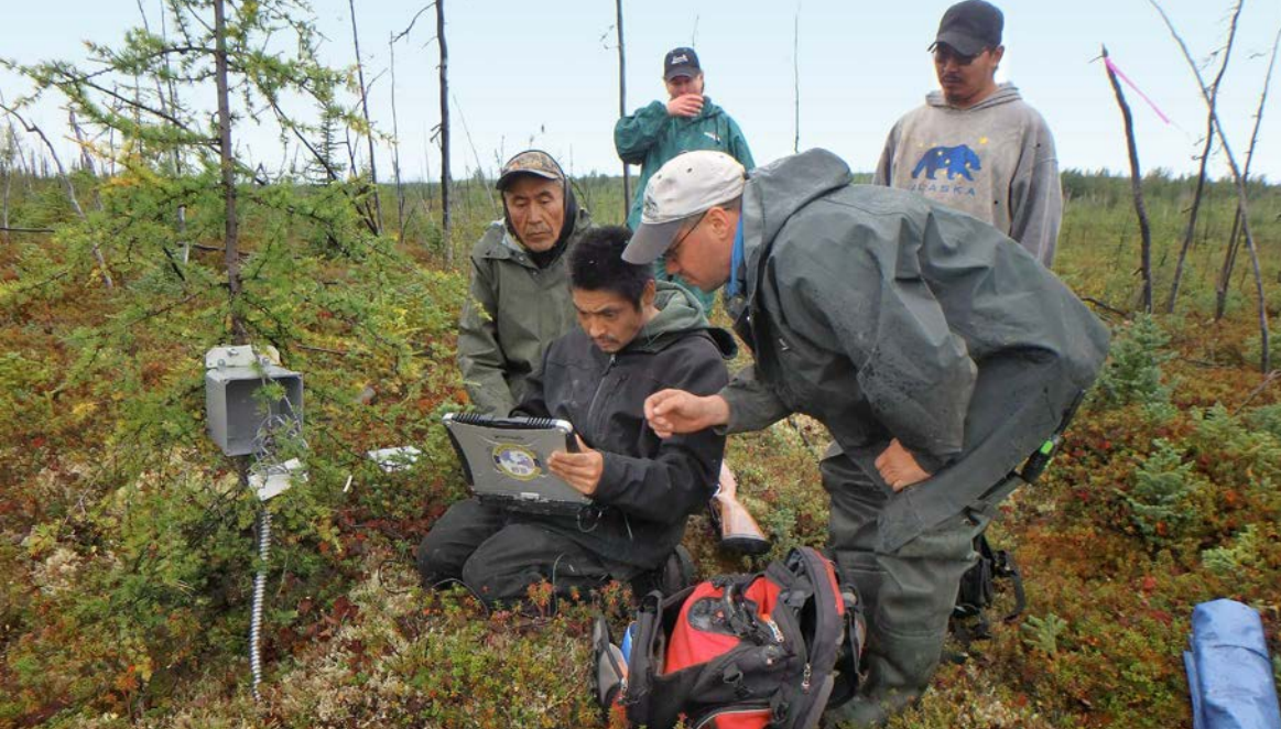
← Installation of soil temperature data logger for NSF sponsored Arctic field programme. © University of Alaska Fairbanks/Santosh K. Panda
