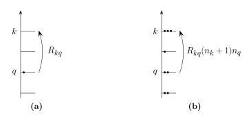
**Figure 2.2.:** Sketch of the dynamics of the occupations in an ideal Bose gas in weak coupling to its environment. (a) For a single particle, the environment induces jumps from level q to k which happen at rate  $R_{kq}$ . (b) Also in the ideal gas, single particles are transferred. The single particle rate for this process is amplified with the occupation  $n_q$  of the departure state and the bosonic enhancement factor  $n_k + 1$ .
