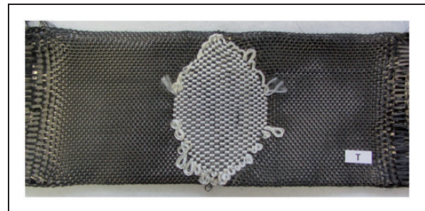
Figure 9. Woven T-structure before erecting (the white yarns are filling yarns).
