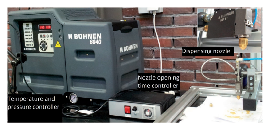
Figure 4. Hotmelt adhesive application device with a dispensing nozzle.
