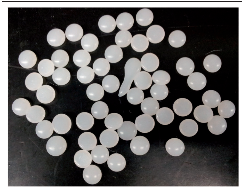
Figure 2. Physical form of hotmelt adhesive.
