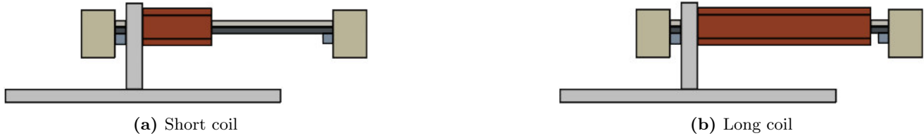
Figure 11: Example of two different long coils, placed at the fixation of the beam
