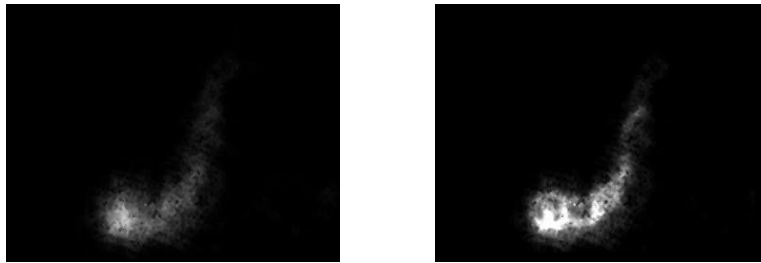
Figure 6. (a) Uniform illumination and (b) HiLo image of zebrafish thyroid.
