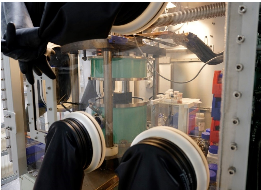
Figure 2.3. Sintering setup Fuji SPS-515S in glove box.
