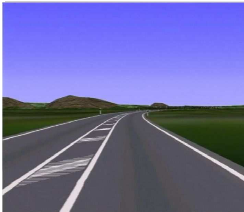
C15 Curve with hatched markings (inbound direction)
