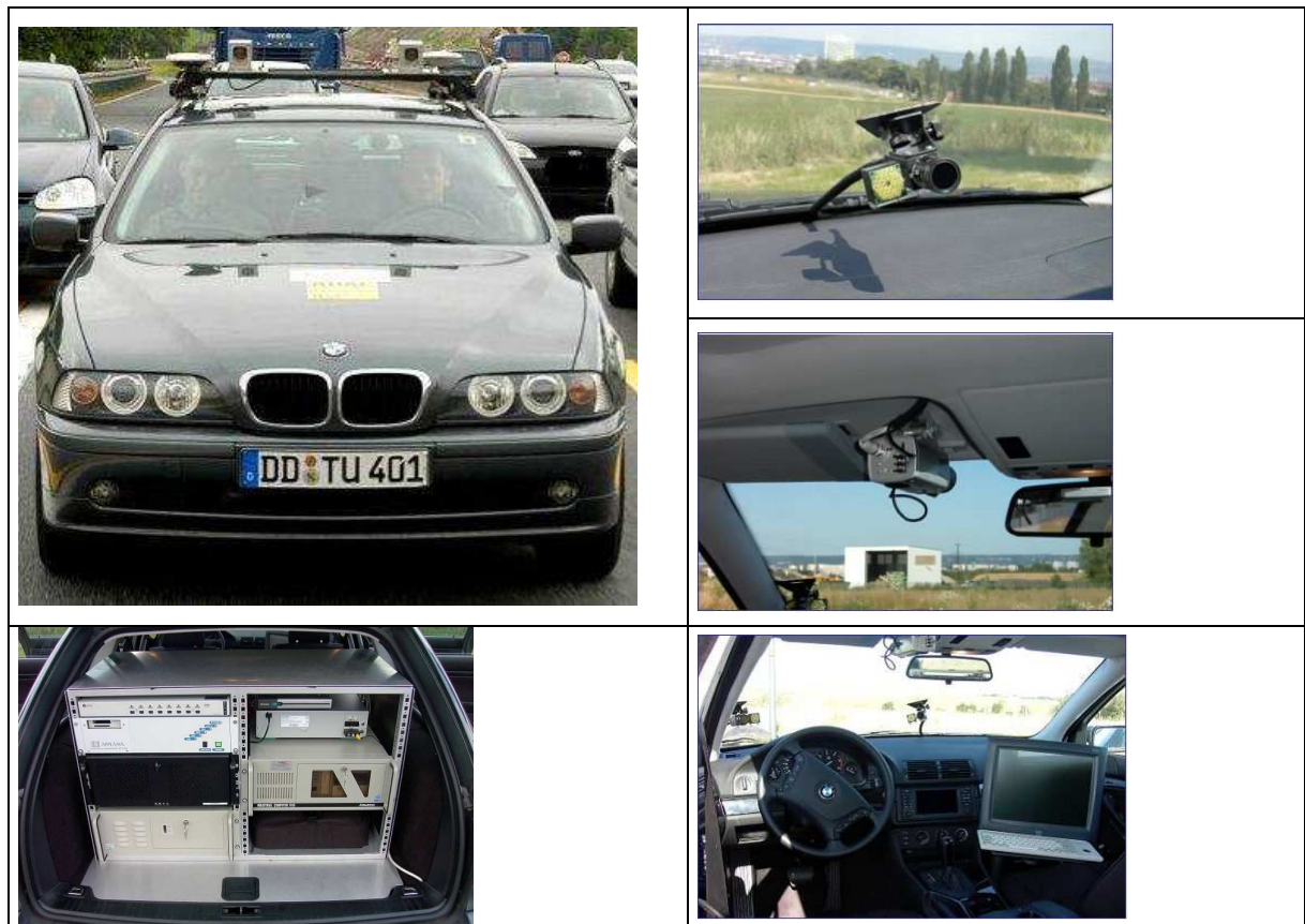
Figure 35. Experimental vehicle of the Chair of Road Planning and Road Design at TUD (Prof. Lippold).
