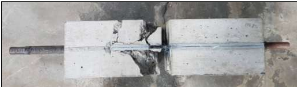
Fig 8. Concrete failure pattern of RTE and RTF
