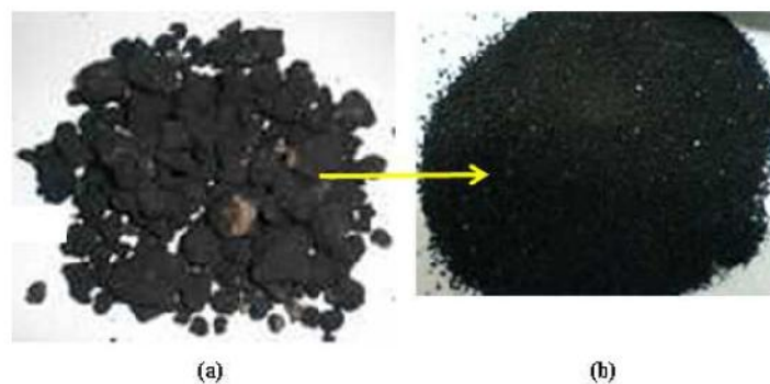
Fig. 2. (a) Particles of BNRA (b) Cruched BNRA diameter 0.15 mm
