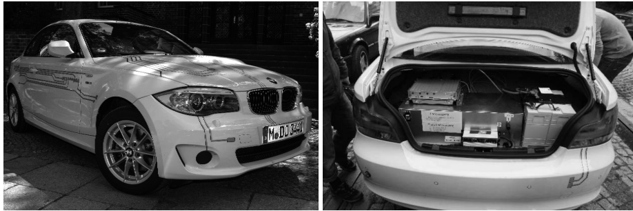
Figure 5: Experimental Vehicle with in-vehicle measurement system.
