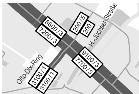
Figure 1: Part of a traffic volume map (format: daily traffic / percentage of heavy traffic).
