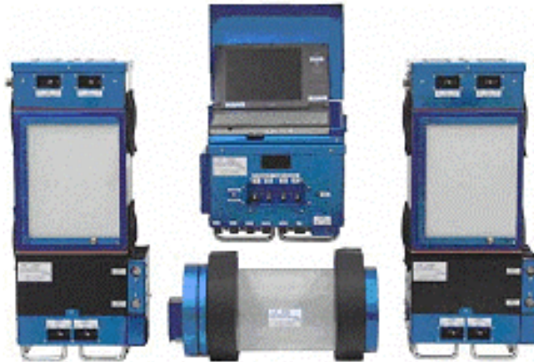
Figure 2-16: Lada; control and display module (upper center), growth modules (left and right), water tank (bottom center) (Bingham et al. , 2002).
