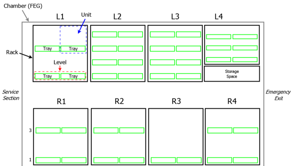
Figure 2-29: Future Exploration Greenhouse – Plant tray configuration including illustration of the relevant definitions of chamber, rack, unit, level and tray (Zabel et al. , 2016b).
