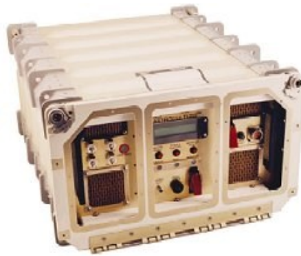
Figure 2-14: ASC-8 flight hardware installed in a middeck locker (Musgrave et al. , 1997).
