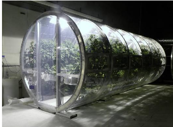
Figure 2-25: Deployed Configuration of the LGH during a test period (Sadler et al. , 2011).
