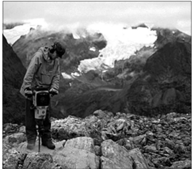
Drilling shallow boreholes for ground temperature monitoring in mountain permafrost in Møre and Romsdal, western Norway, September 2002. (Photograph provided by Ketil Isaksen.)
