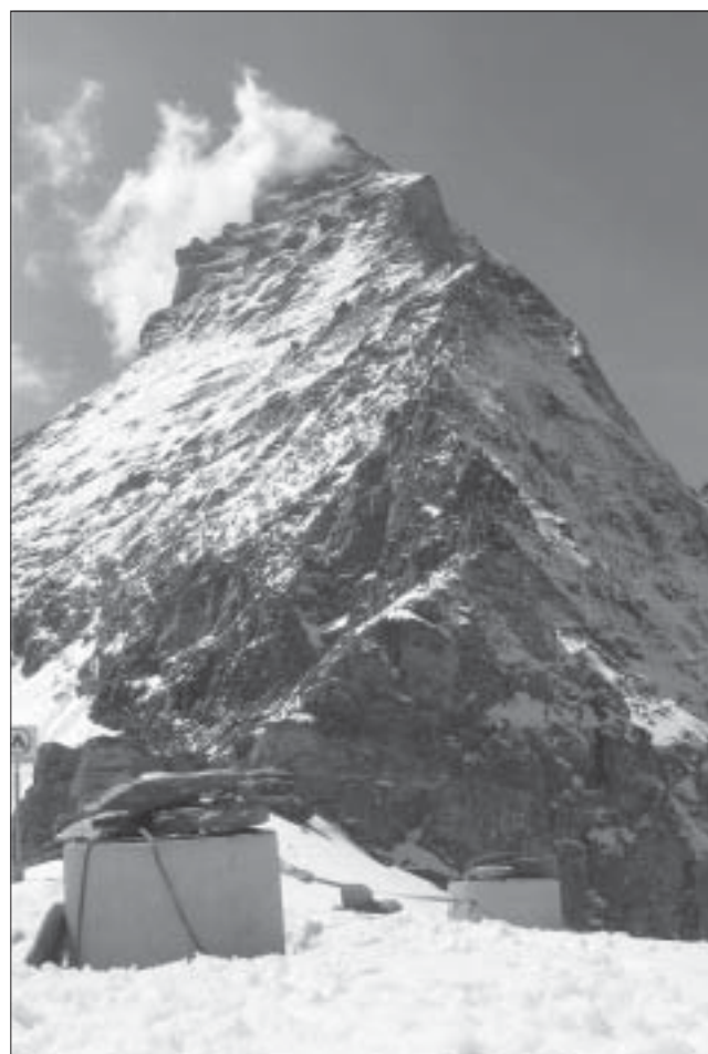
Two 60 m vertical boreholes instrumented with thermistors in the Matterhorn Hörnli ridge at 3300 m asl. Photograph by M. Philips, August 2006.
