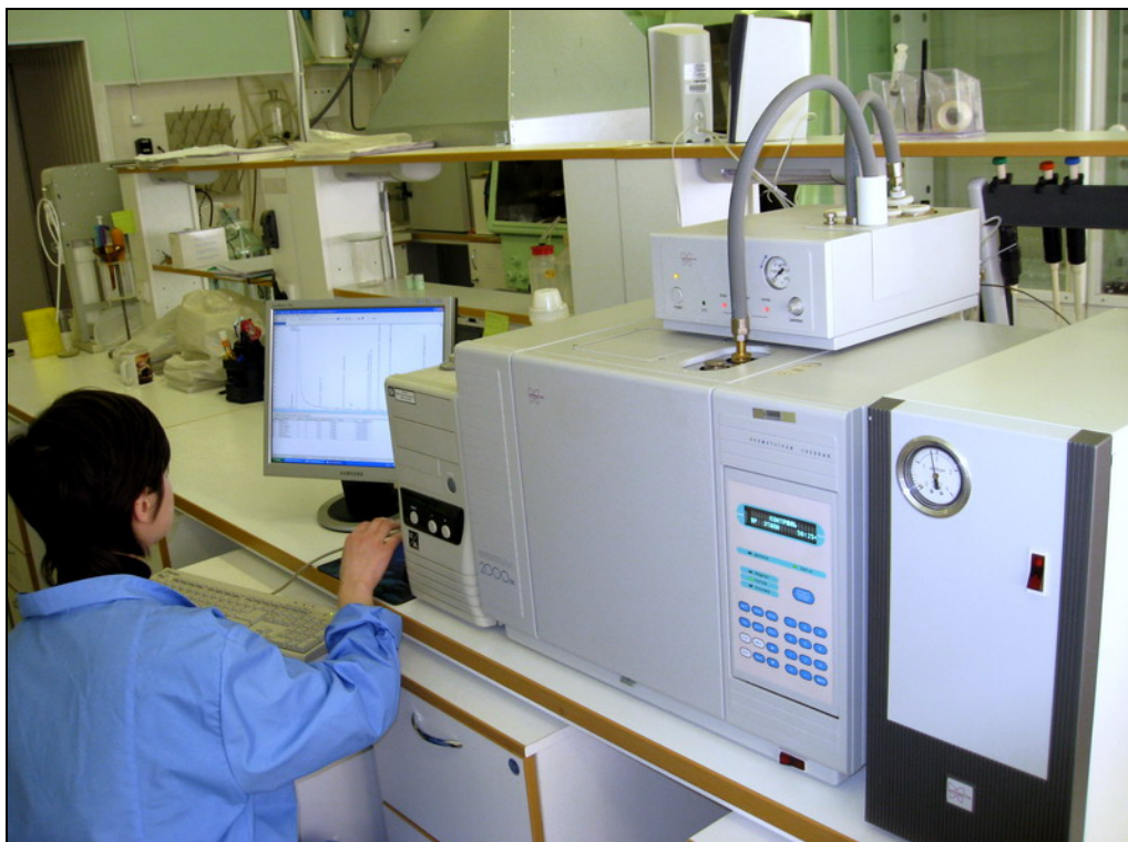
Figure 5.2-6 VAH analysis at the chromatographic analytical system based on gas-liquid chromatograph “Kristall-2000M” with a flame ionization detector
