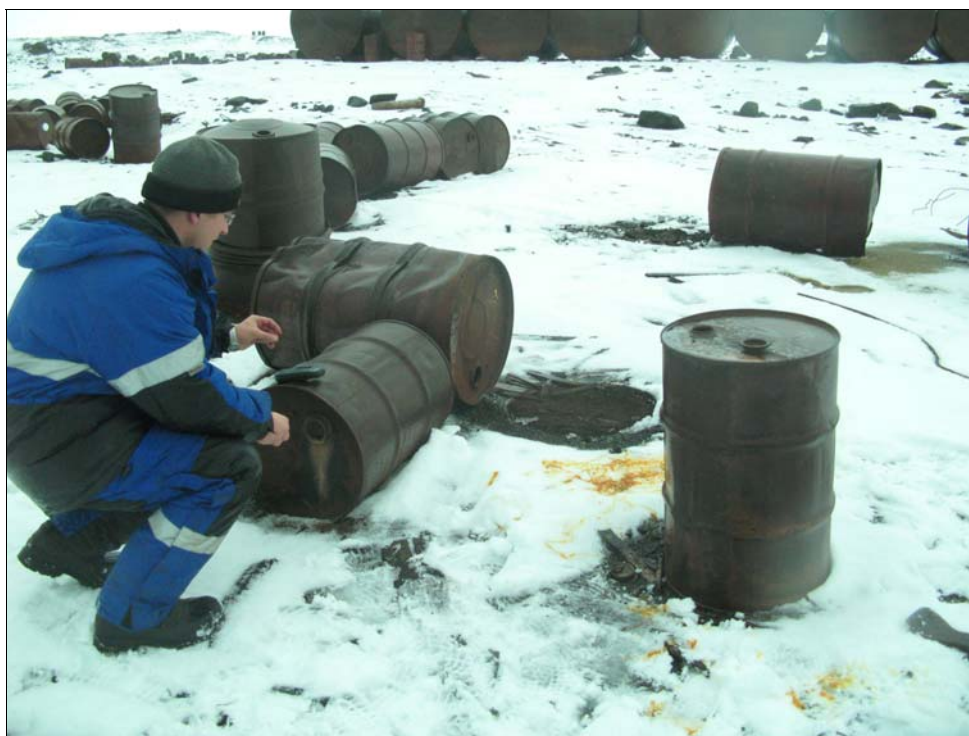
Figure 5.4-4 Collection of technical liquid specimens at site 1 (fuel and lubricant storage facility in Severnaya Bay), Alexandra Island
