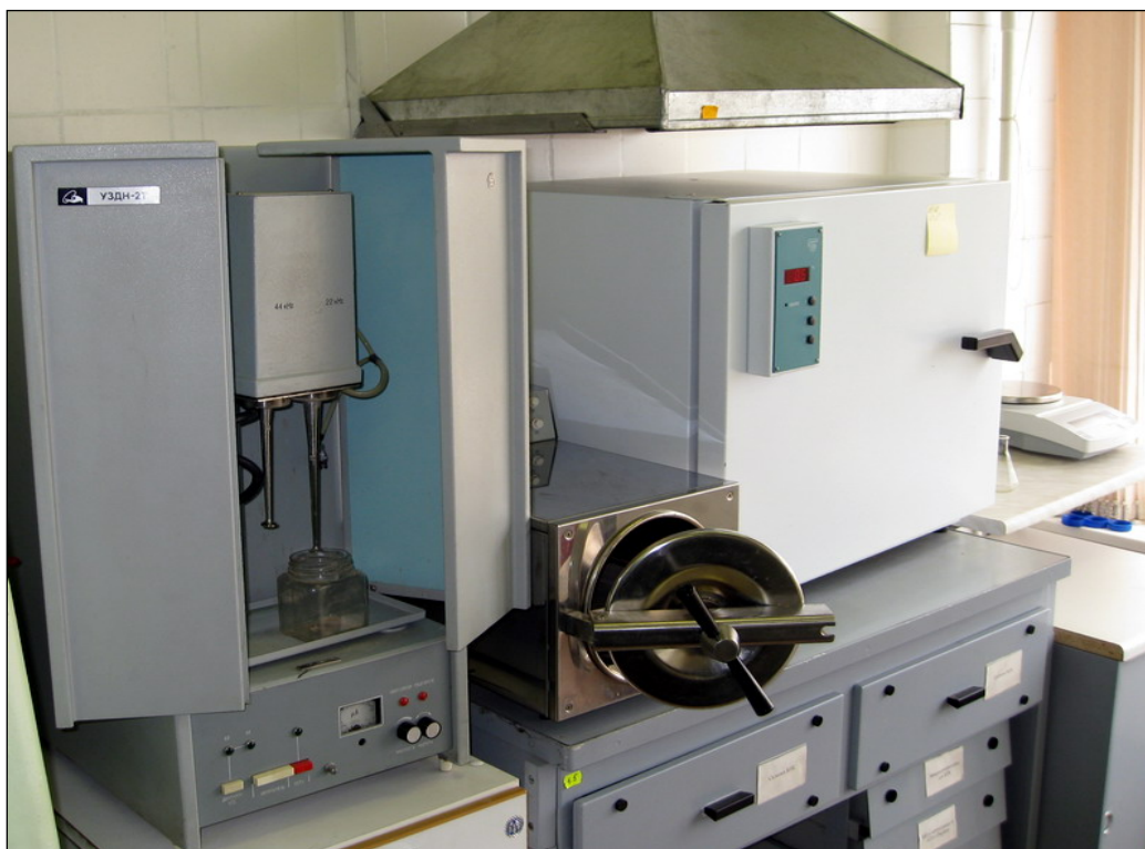
Figure 5.2-9 Atomic absorption spectrophotometer A-02
