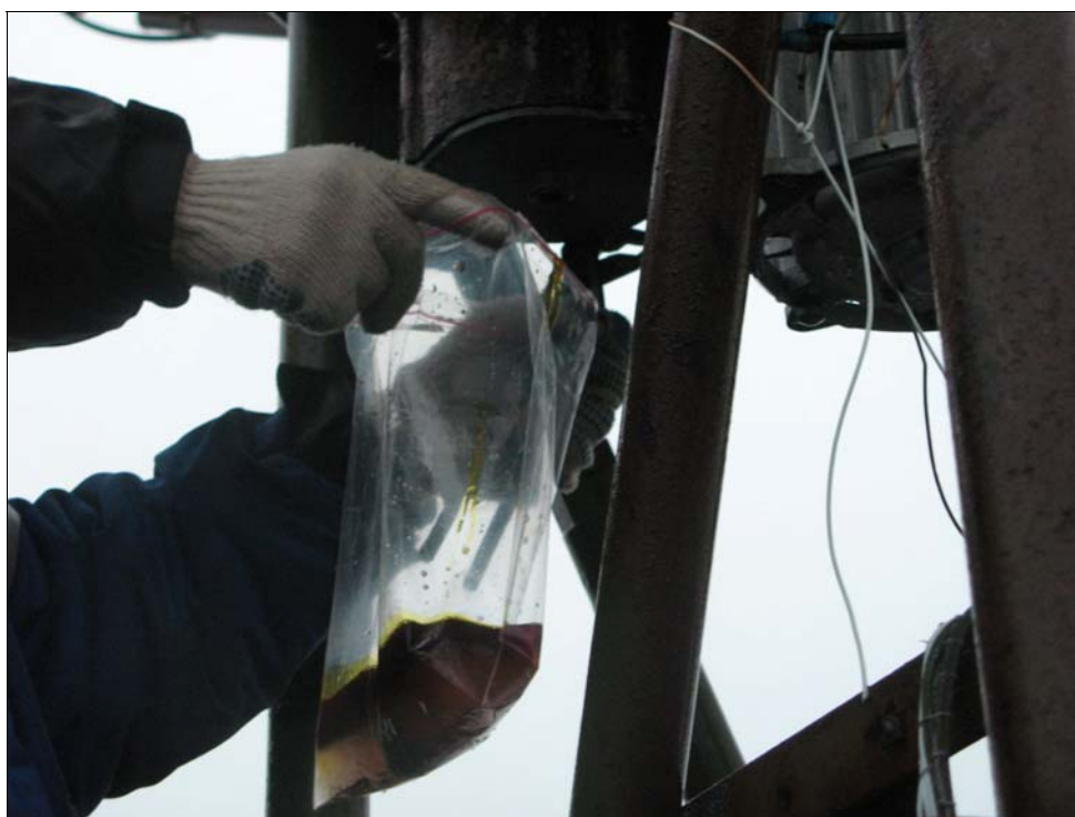
Figure 5.4-1 Collection of a technical liquid sample from a radar transformer at site 9 (radar station), Alexandra Island
