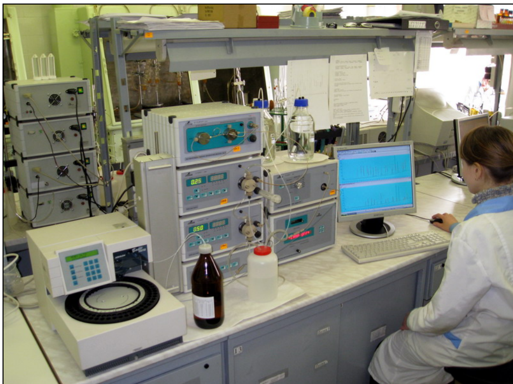
Figure 5.2-5 PAH analysis at chromatograph analytical system based on gradient liquid chromatograph “Stayer Gradient”, autosampler Stayer Basic and UV and fluorimetric detectors
