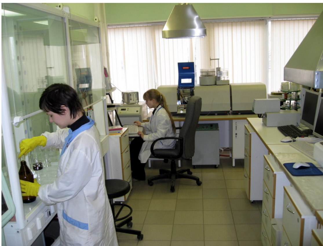
Figure 5.2-8 Heavy metal analysis with the use of an atomic absorption spectrophotometer A-02
