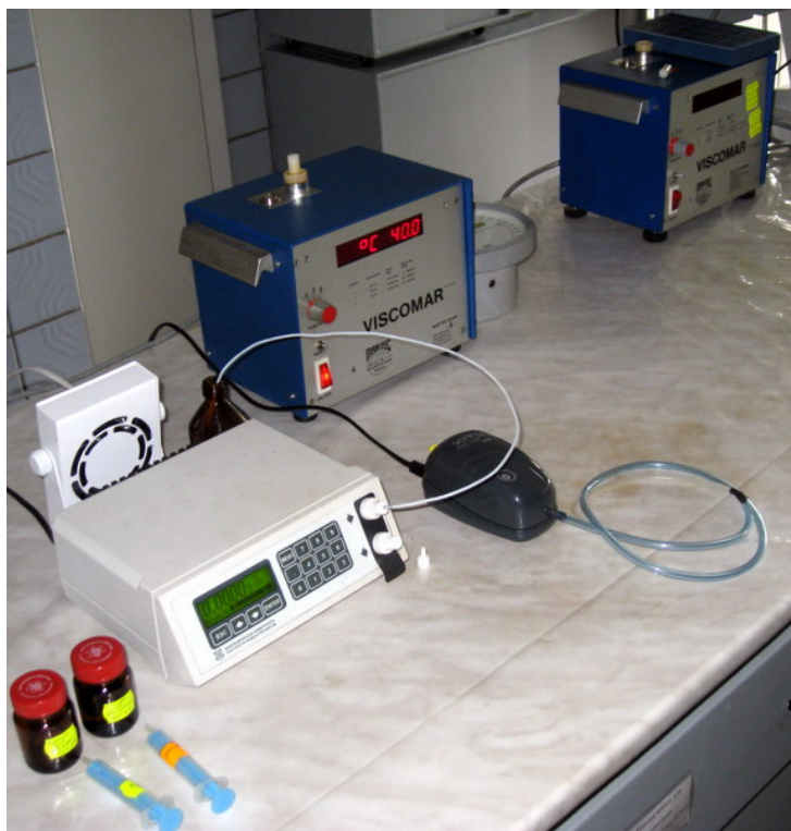
Figure 5.2-14 Digital density and viscosity meters for oil products
