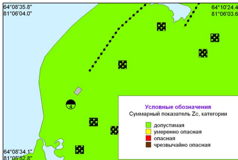
Figure 5.3-35 Spatial characteristics of the level of soil contamination of the drum storage facility on the coast area (site 5) with a series of heavy metals (Zc)
