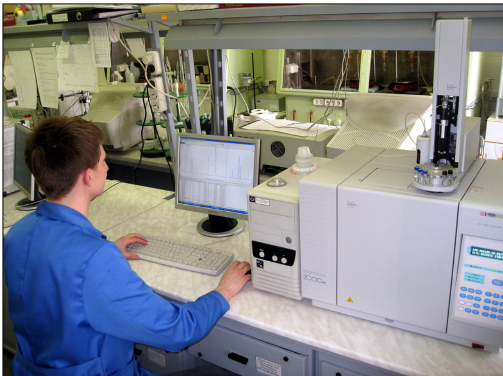
Figure 5.2-2 PCB analysis with a chromatograph analytical system based on gas-liquid chromatograph “Kristall-2000M” with electron capture detector
