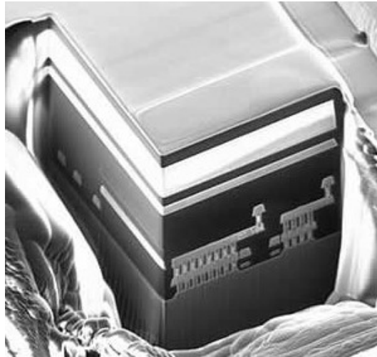
Fig. 2.4 SEM image of two perpendicular cross-sections of an Integrated Circuit done with FIB[43].
