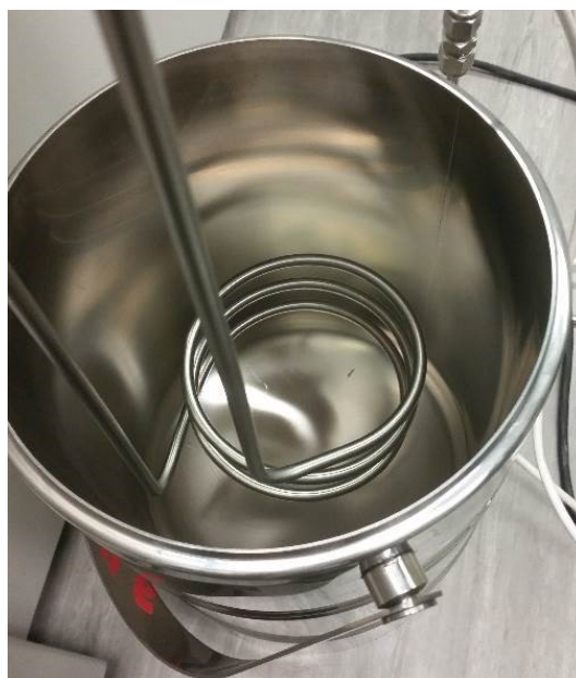
Fig. 4.5 Liquid nitrogen cold trap (LNCT) with a Dewar flask and a spiral pipeline going in and out of the flask.
