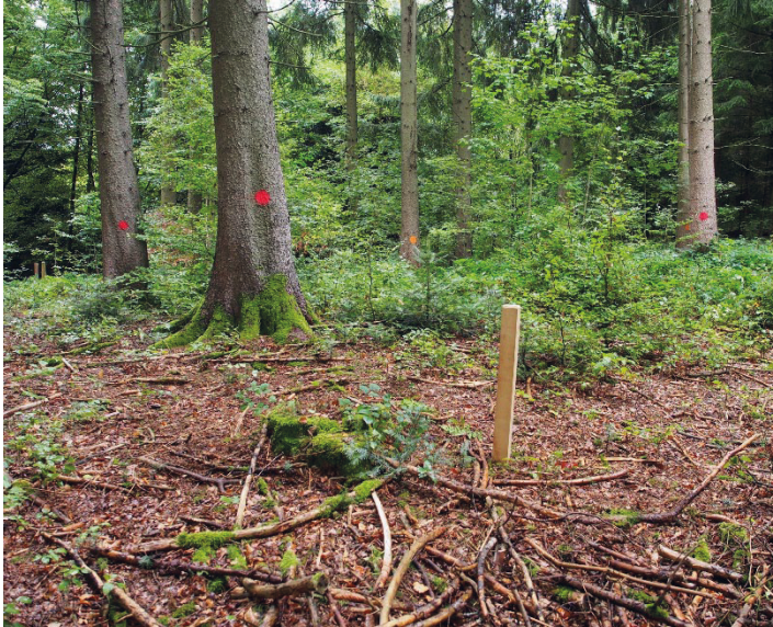
Figure 4: One of the training plot for basal area measurement with the Bitterlich method (trees with red circle to be counted with a counting factor of 4, trees with orange circle with k=2 ).
