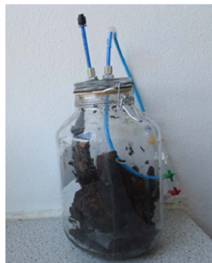
Figure 2. Test kit for determination of CH 4 removal capacity
