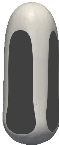
Fig. 5.5 Location of the thin film area (dark regions) on a Taylor bubble surface in a square channel.
