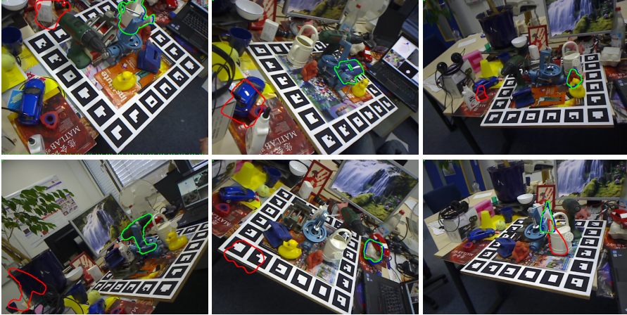
Figure 4.7.: Results - Global Hypothesis Generation. Qualitative results on the “Occluded Object Dataset” [8]. Results of our method are depicted as green silhouettes, the ground truth pose is shown as a blue silhouette and results of the method by Krull et al. [64] are shown as red silhouettes. Note, since these results shows correct poses of our method the green silhouette is on top of the blue one.
