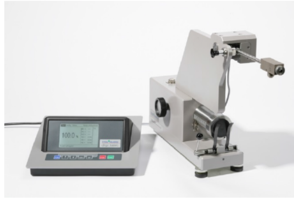
Figure 3.10 Free fall pendulum based rebound resilience tester
