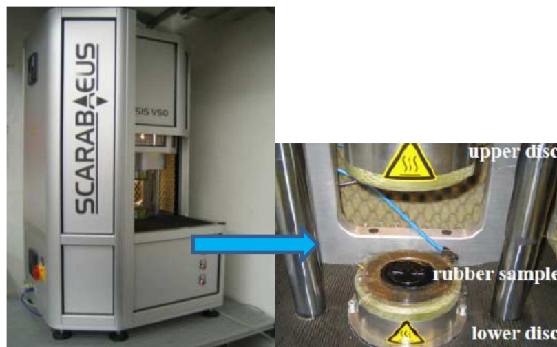
Figure 3.5 Rubber process analyser for the determination of processing characteristics
