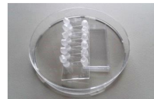
Figure 15: Tilted chamber position during degassing
