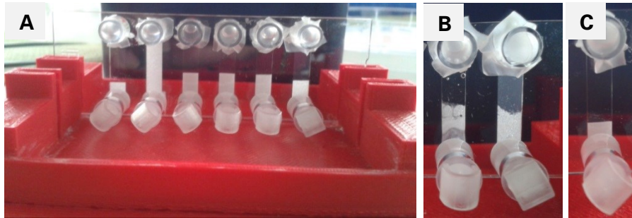
Figure 13: A ) Position of chamber in holder before baking. B ) First channel is unusable as the bottom part is melted together completely after baking (indicated by transparent appearance). The second channel is ok, but a few beads are in the channel above the stack. C ) Perfect channel with no beads in the channel after baking.
