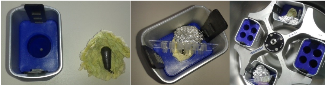
Figure 11: Centrifuge preparation. Place the lead in tissue paper into the tube holder, position the chamber on the tube holder with outlets at the bottom and stopper/reservoirs facing outwards. Take care that the holders are properly inserted into the centrifuge.
