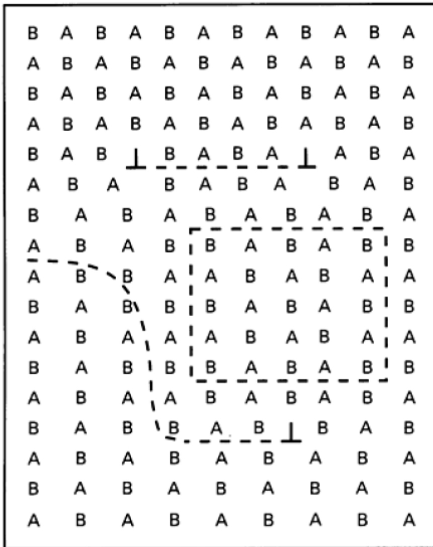
Figure 2.5 Schematic representation of 2-D simple cubic lattice containing a super-lattice dislocation (paired dislocations) and two antiphase boundaries [Sto66].
