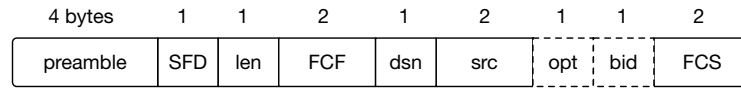
Figure 7.5: The format of a beacon for responding to a neighbor discovery request.
