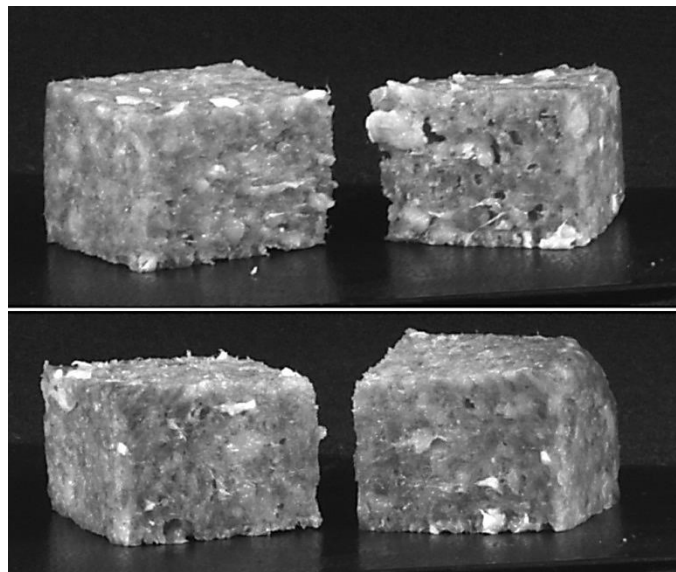
Figure 5.18: Surfaces of Salami after cutting at 10^{-1} m/s (rough, upper picture) or at 10 m/s (smooth, lower picture).
