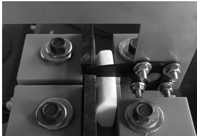
Figure 4.8: Sample support rig with a bubble gum sample (white) and blade (black) support of the universal testing machine for multi-scale cutting velocity experiments.
