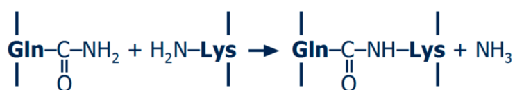
Figure 2. Reaction scheme of protein polymerisation by transglutaminase.
