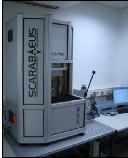
Figure 3.4 Rubber process analyzer: moving die rheometer (Scarabaeus SIS V50)
