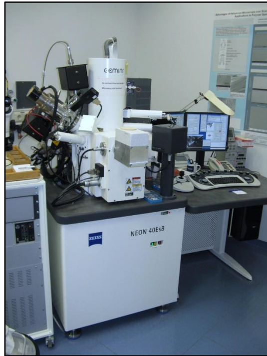
Figure 3.6 Scanning electron microscope (NEON 40 EsB) by Carl Zeiss
