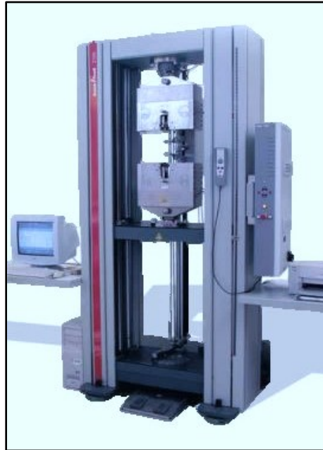
Figure 3.7 Universal testing machine (Zwick 1456, Z010) by Zwick/Roell AG
