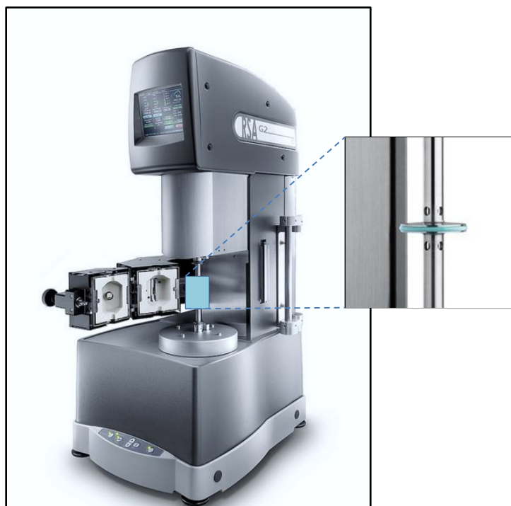
Figure 3.3 ARES-G2 Rheometer showing parallel-plate test geometry [ http://www.tainstruments.com/ares-g2/ ]
