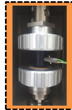
Figure 4.40 Curves of flexometer test. The final surface and core temperatures of specimens are as inset table. The core temperature is measured by using a thermocouple, as is shown in a photo of flexometer test setup.
