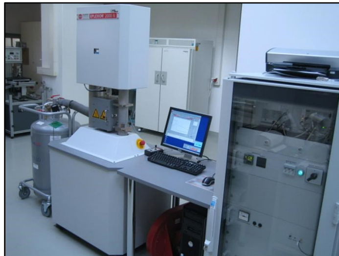
Figure 3.8 Dynamic Mechanical Thermal Spectrometer (Eplexor 2000 N) by GABO Instruments
