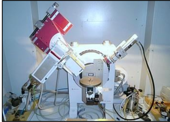
Figure 3.9 X-ray Diffractometer (XRD 3003 T/T) by GE Sensing & Inspection Technologies
