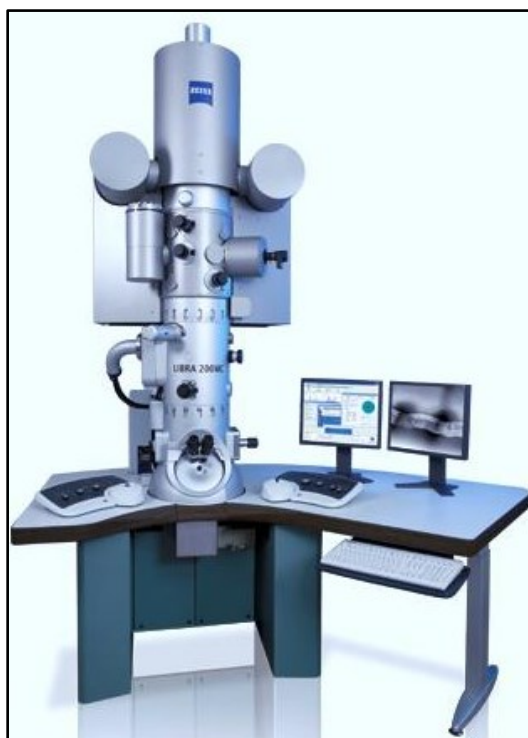
Figure 3.5 Transmission electron microscope (Libra 200 MC) by Carl Zeiss
