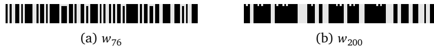
Figure 6.5.: Space-Time-Diagrams of w_{76}, w_{200} with random initial condition and periodic boundary, black represents 0 and gray represents 1.
