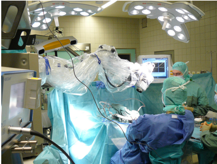
Figure 1.2.: Recent developments have enabled parallel thermal and optical imaging by adapting the thermal camera to an OP microscope.
