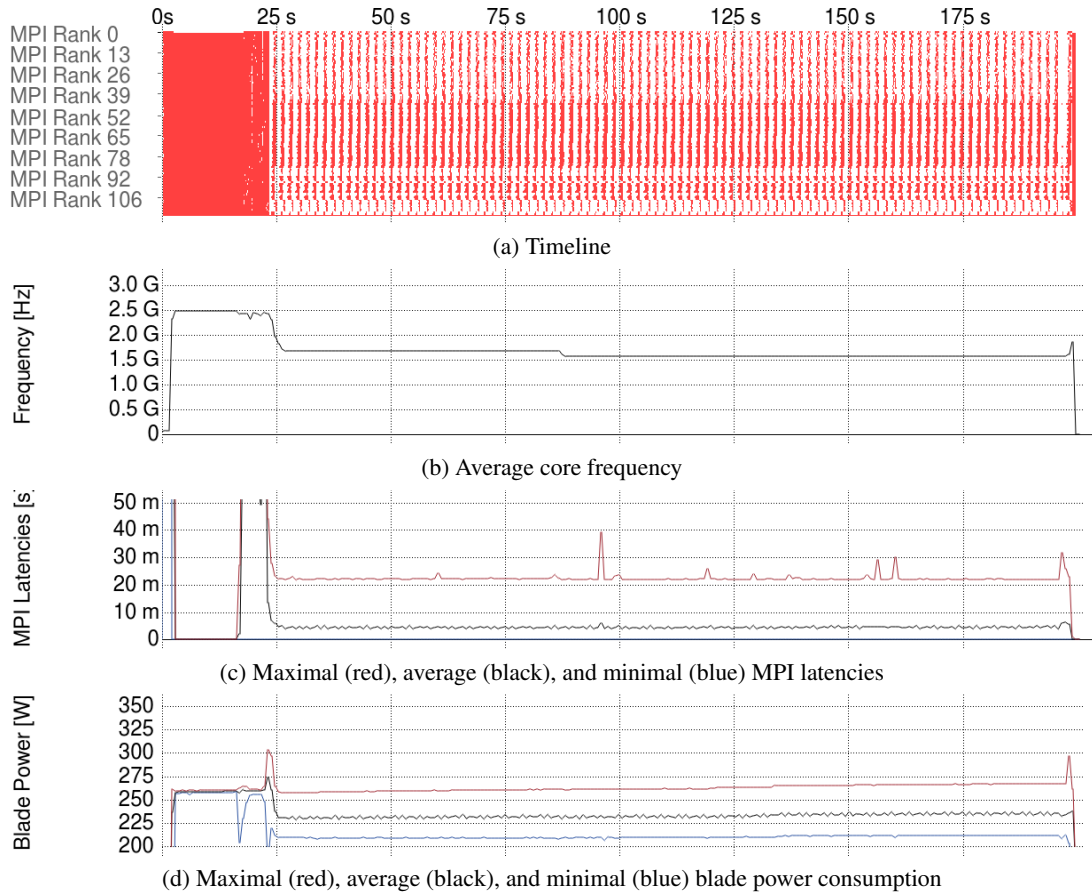
Figure 7.13: Vampir visualization of an optimized run of the SPEC MPI2007 benchmark 113.GemsFDTD (medium reference input set). MPI latencies, some processor frequencies and the average power consumption decrease, while the runtime is extended.
