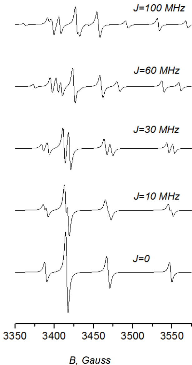
Figure 3.17. Simulated EPR data for the biradical particle with different values of spin-spin coupling constant J . other EPR parameters such as a_{\perp}(^{89}Y)=74,3 G (208 MHz) and a_{\parallel}(^{89}Y)=87,8 G (246 MHz), g_{\perp}=1.9620 , and g_{\parallel}=1.9982 are fixed.
