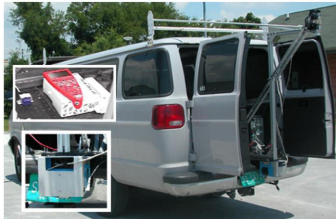
Figure 1. The prototype of mobile mapping system composed of laser scanner (bottom inset) and video camera, and GPS/IMU (top inset) (Yu, et al., 2007)
