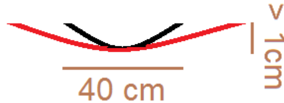
Figure 61. Schematic view of the curvature difference between two ruts (shown in red and black)
