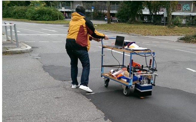
Figure 100. An example of training data collection from a new asphalt section by Polytec spectrometer
