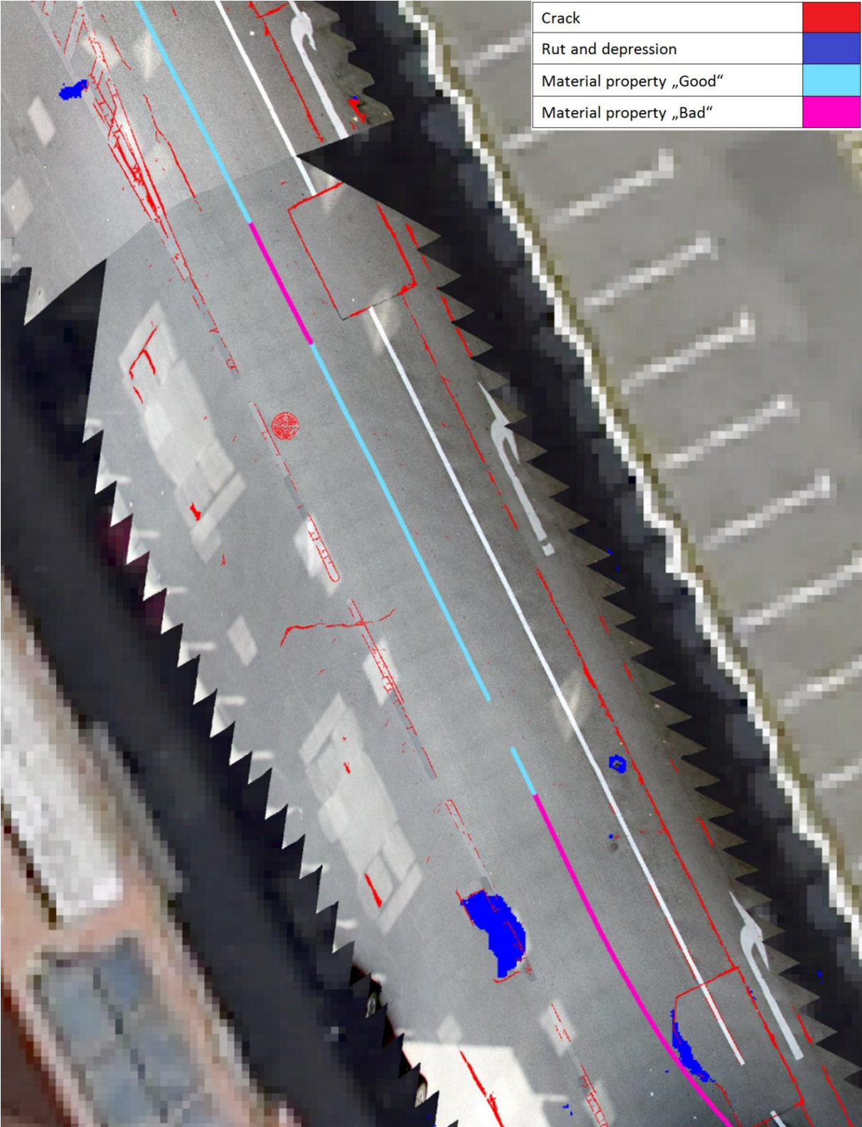
Figure 106. Second sample of road section containing integrated pavement distresses and the result of asphalt quality classification
