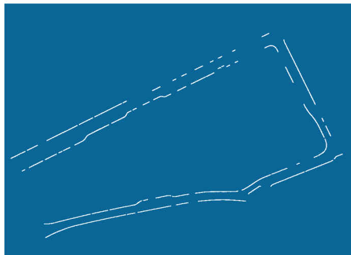
Figure 44. Filtered result of potential road boundaries by means of area and roundness as geometric properties of the potential road boundary regions
