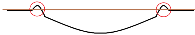
Figure 54. Schematic representation of peaks on rut support (uplifting of the sides of a rut)
