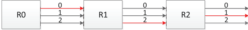
(b) In this SDM NoC, each link is split into 3 sub-channels. Along the path, if sub-channel 0 is reserved in R0, any free sub-channel can be reserved at the next hop.
