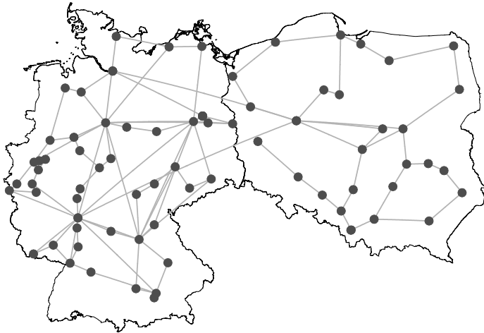
FIGURE 3.5: NREN topology in Germany and Poland. The illustration of two connected NRENs in Germany and Poland consists of 82 nodes and 116 links in total.
