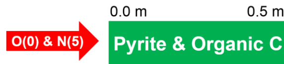
Figure 17 Schematic 1D model. The column is characterized by oxidized zone with nitrate and oxygen and lower reduced zone with pyrite and organic carbon.
