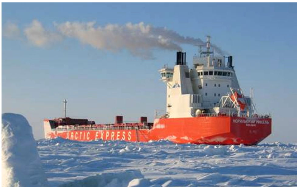
Icebreaking (Double Acting) Container Ship: Norilskiy Nickel on the Northern Sea Route (March 2006)
