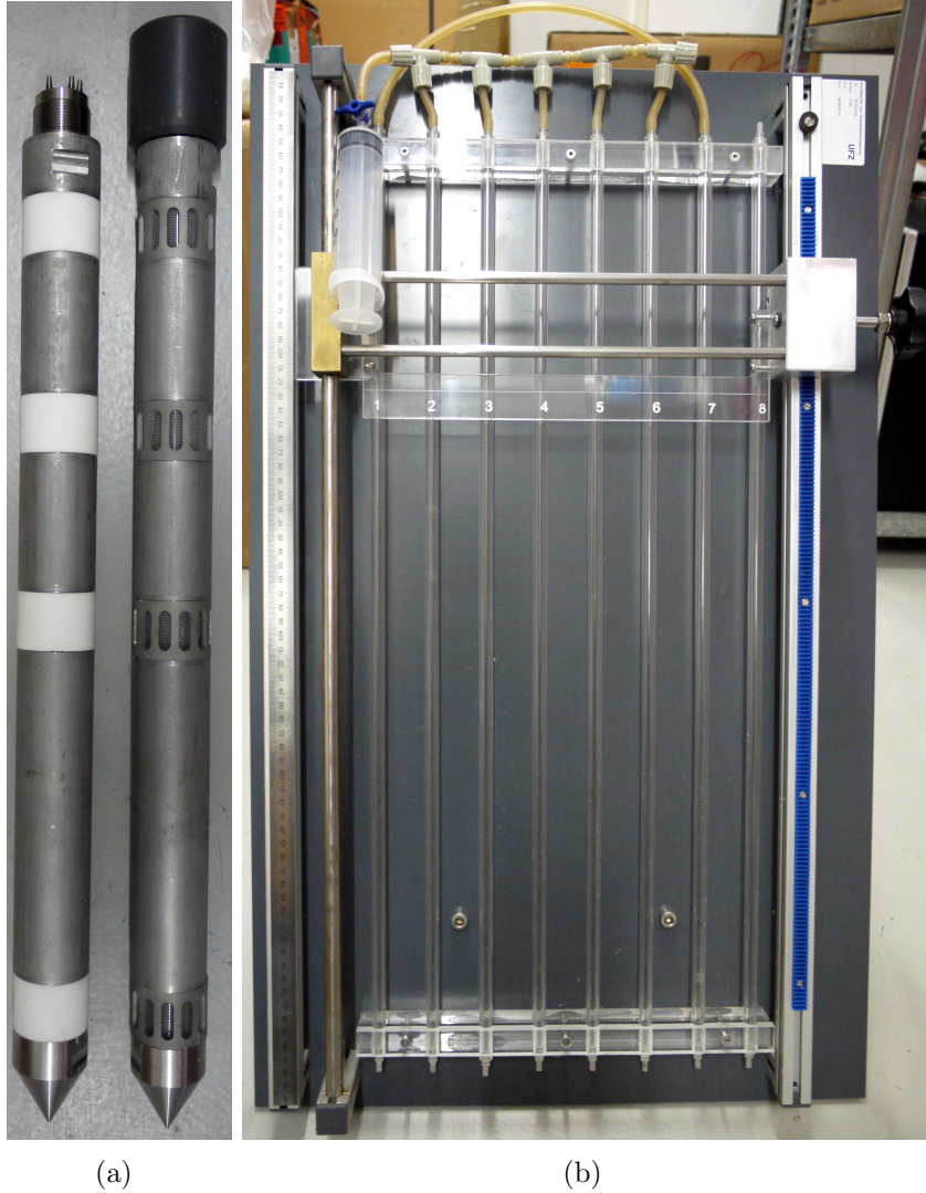
Fig. A.5. – Multi-level sampler (after Lenk et al. (1999)) (a); white plastic filter were used in order to prevent clogging of the pipes; a teflon tube was attached at each of the pipes that come out on top of the sampler. The tubes can either be connected to a syringe for sampling of the subsurface water or to a pressure-meter (b) in order to check the vertical hydraulic gradient at each sampling depth.
