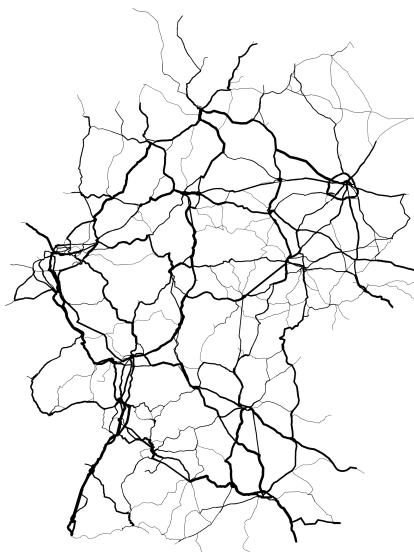
Figure 1.1: Real-world instance of Germany's long-distance train path system depicted as infrastructure network with corresponding capacity utilization (screenshot of software system TAKT).
