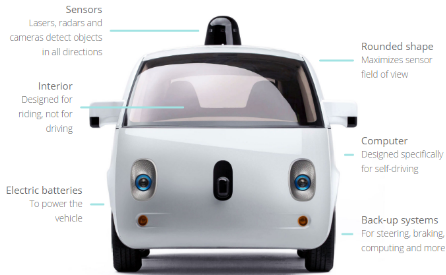
Fig. 3. The Google car with its main components shown from the front, as presented on the official project page.
