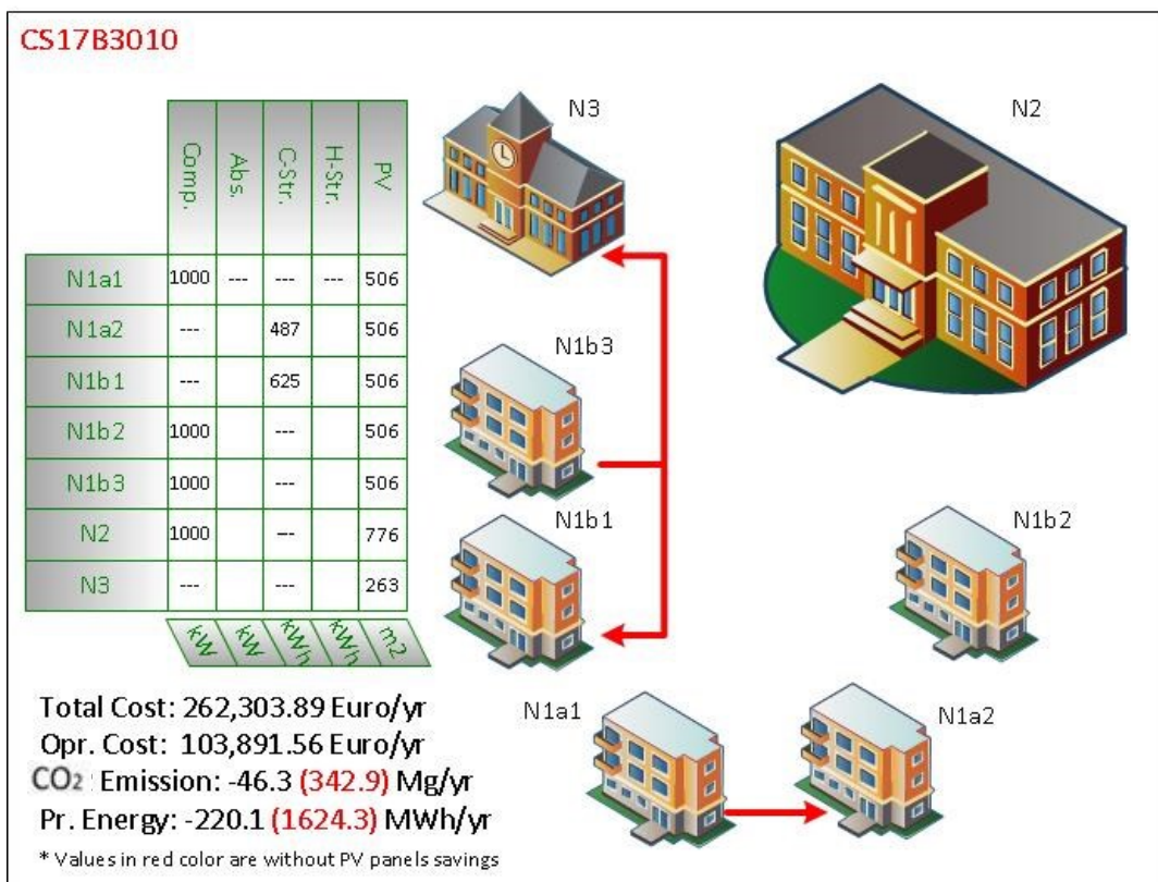
Figure 4.79: De-centralized DC network scenario at Multi objective (cost 1-1 CO 2 ) optimization stage for case study 1 with electricity tariffs A and B.
