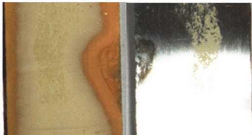
Fig. 4.25: Bondline corrosion detected on a Smut-Go NC pickled AA 2024 clad specimen after only 15 d exposure to mere hot-wet conditions (35 °C, 100 % rh)
