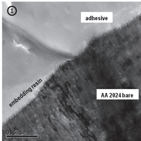
Fig. 4.39: TEM image of the delamination front of a GPS plasma coated AA 2024 bare ( \text{HNO}_3 ) adherend after bondline corrosion test
