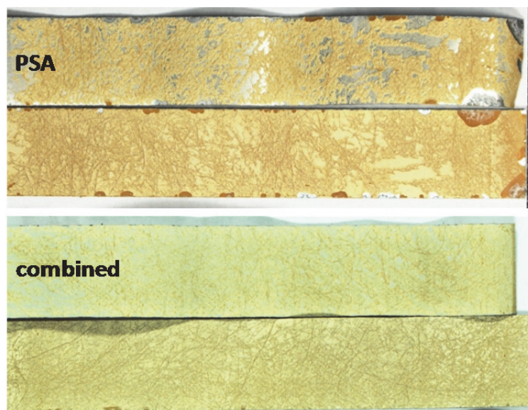
Fig. 4.60: Exemplary AA 2024 clad bondline corrosion test coupons (FM 73) after 30 d SST
