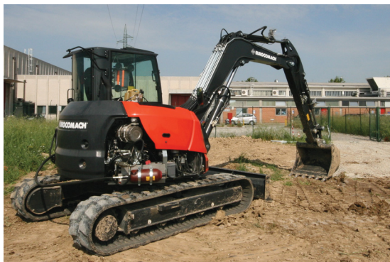
Figure 8: Hydraulic Hybrid Excavator Prototype on the Testing Field
