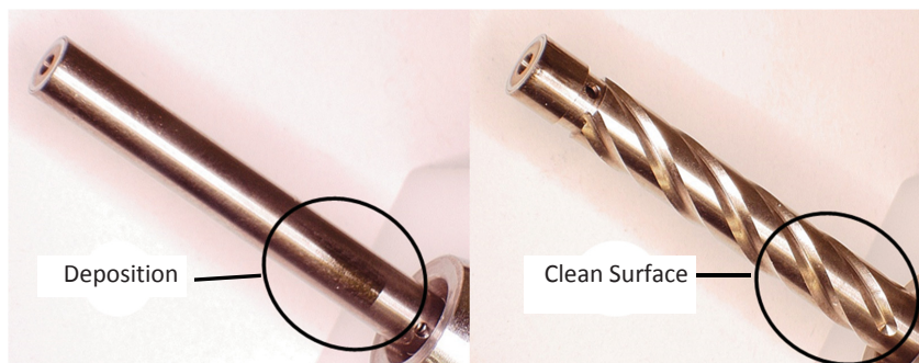
Figure 13: Effect of helix grooves at the piston (right) after durability test
