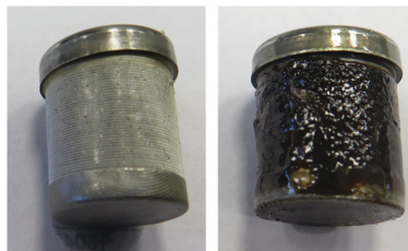
Figure 11: Example of deposits originating from degenerated biodiesel B20
