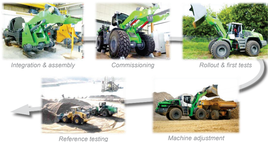
Figure 5: Integration, commissioning and testing of the „Green Wheel Loader“
