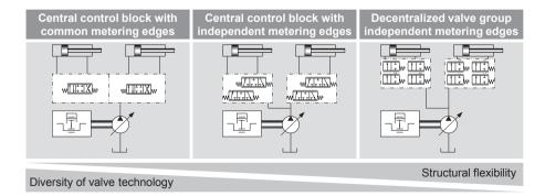
Figure 11: Individualization levels of valve controlled actuators
