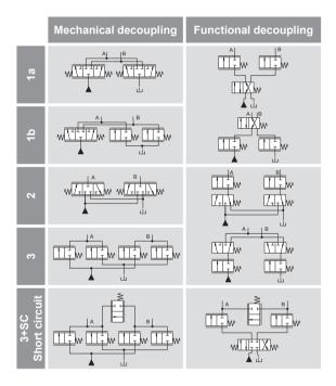
Figure 12: Different variants of valve structures
