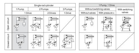
Figure 3: Pump control of a single rod cylinder, general (left) and in particular with one pump (right) /10/
