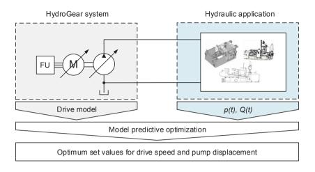
Figure 4: Model predictive optimization of HydroGear systems
