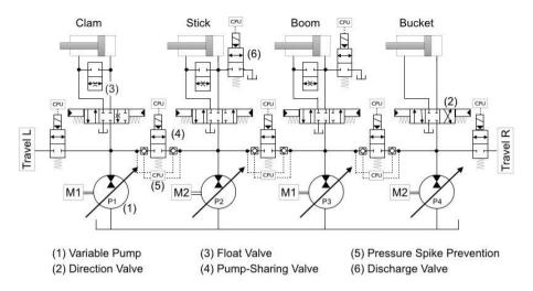
Figure 10: Circuit diagram of a 290 t mining excavator
