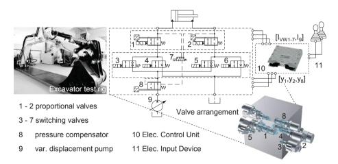
Figure 19: Test rig setup
