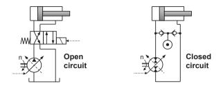
Figure 7: Basic concepts of displacement control
