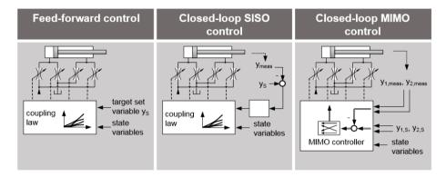
Figure 15: Control architectures of independent metering systems
