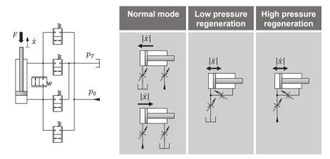
Power consumption of IM over conventional directional valves assuming the same supply pressures (Single-rod cylinder with area ratio 2:1)
