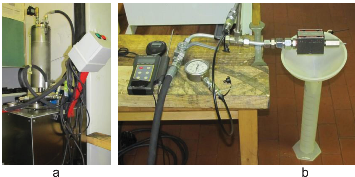
Figure 12: Water hydraulic test rig. a) power pack. b) tested valve
